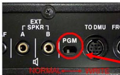
Carefully move the PGM-SW on the SM-5000 to the **WRITE** (program position).
