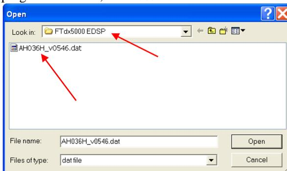
**NOTE:** If you receive a “Communications Error” message on your screen you should check the COM port number and speed under Device Manager. The writing speed **38.4kbps** is fixed in the download algorithm of the EDSP board so you may need to set the port speed close to 38.4kbps. Click on the **COM Select** box arrow and choose a different COM port from the drop down menu in the EDSP-5000 writer. Please refer to page 4 for additional details.
