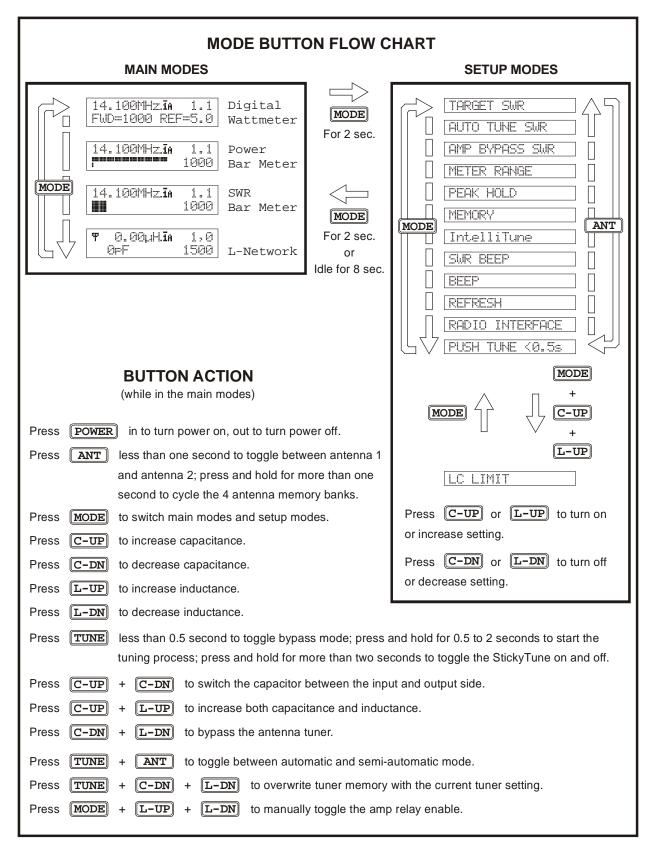
Figure 3. Mode Button Flow Chart and Button Action.
