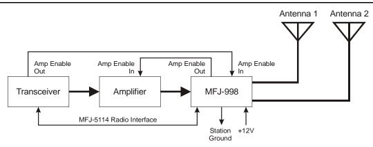
Figure 1. Typical Installation Block Diagram.
