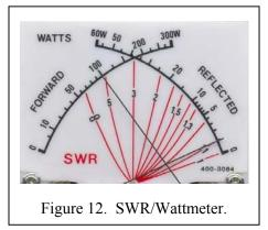
The meter can be set to low, high, or auto range (default). Auto range automatically sets the meter scales according to the input RF power to the tuner. Forward power greater than 300 watts or reflected power
