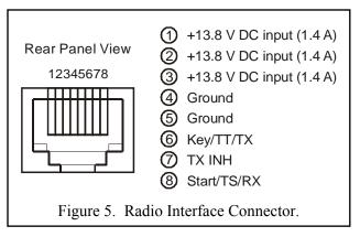
The Radio Interface works with radios that are compatible with Alinco EDX-2, Icom AH-3 and AH-4, Kenwood AT-300, and Yaesu FC-30, FH-1 and FH-2. When connected to a compatible radio, simply press the [TUNER] or [AT] button on the radio; for FH-1 or FH-2 compatible Yaesu, press the [TUNE] button *on the tuner* to start the automatic tuning process. The radio will automatically switch
