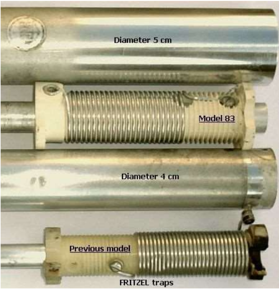
Top: Fritzel model 83 trap, Bottom: arcing and damage in a 1970/71 trap.
