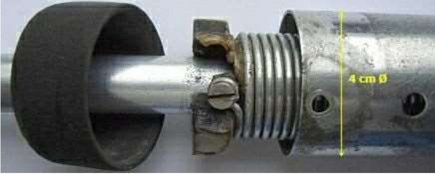
Damage due to a dirty (vintage) trap and power exceeding.
